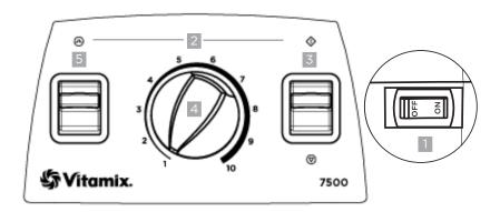
1. **On/Off Switch:** The On/Off (or Power) Switch is on the right-hand side of the machine base. The On/Off Switch controls the power to the machine.
