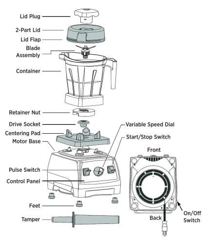
**On/Off Switch:** The On/Off (or Power) Switch is on the right-hand side of the machine base. The On/Off Switch controls power to the machine.
