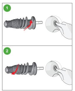
Press [Rev] button for 3 to 5 seconds, then release. When the [Rev] button is released, the auger will stop rotating. Repeat this 2 to 3 times. The [Rev] button pushes the ingredients upward releasing the food clog.
