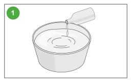
You can thoroughly wash parts by immersing in warm water diluted with one or two drops of baking soda or dishwashing soap for about 30 minutes.
