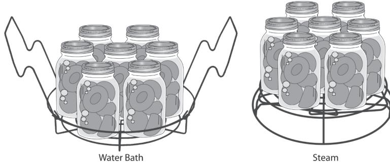
This rack has handles on one side and the other side is flat. For Steam Canning, fold the handles down inside the rack, turn the rack over, and place it in the canner with the flat side up. To use the rack for water bath canning, remove the rack from the canner and pull the handles out, then hook them on the sides of the pot.
