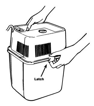
Pull out on the bottom of the latches, **one side at a time.** Release one latch and pull up, then release the second latch.
